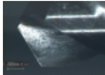
Small wear after drilling 10400 holes
